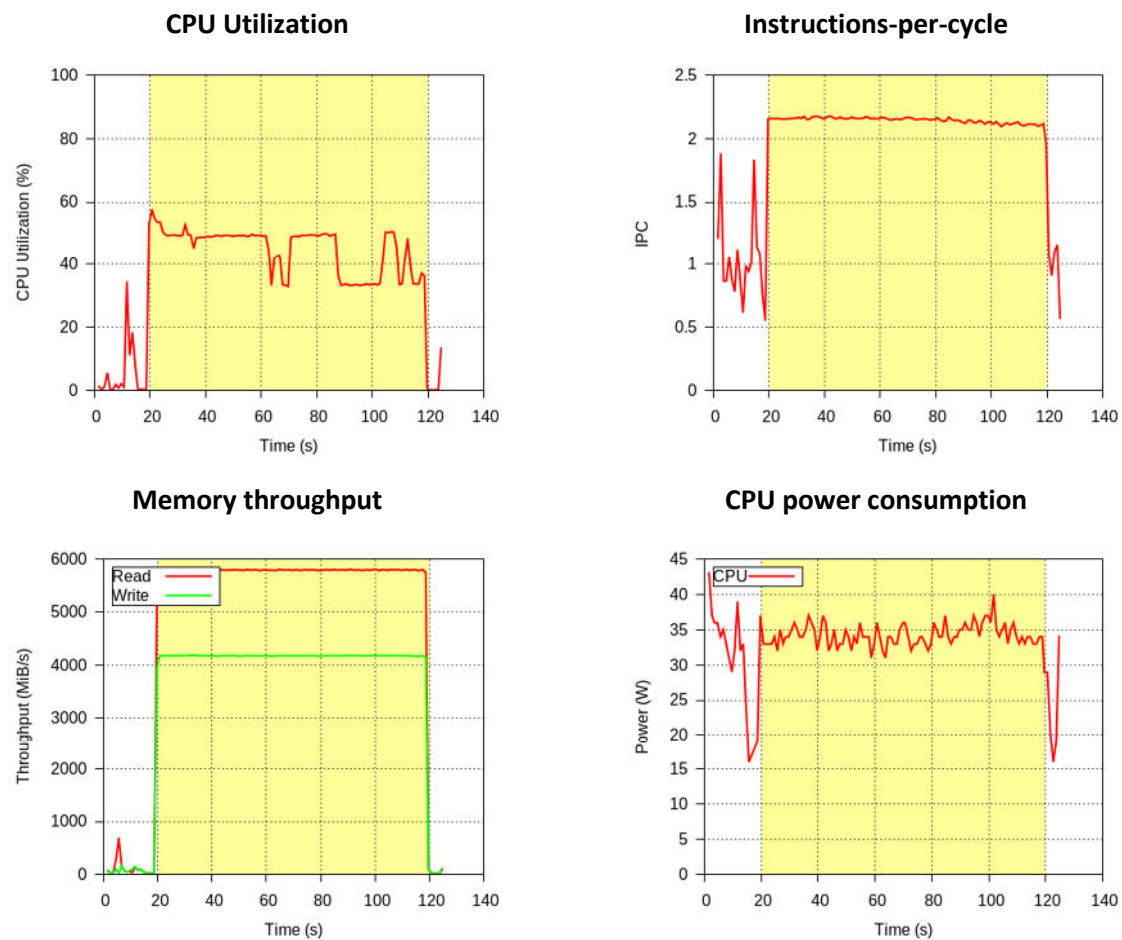
Figure 27 – Example profiling data, covering the most relevant resources for that benchmark
